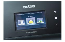
Secure Function Lock (SFL) allows user restrictions to be put in place for function management and improved security.
