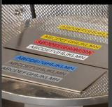
After laminated labels were placed in a fade-inducing chamber to simulate a year in sunny surroundings, the text was unaffected.
