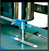
After a 1kg sanding device was passed over the laminated labels 50 times, the text was unaffected.
