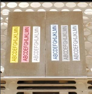
Laminated labels were subjected to temperatures ranging from -80C to +150C for 240 hours, and the text was found to be unaffected.
