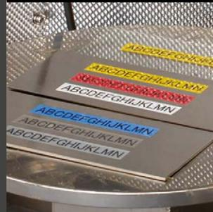
After laminated labels were placed in a fade-inducing chamber to simulate a year in sunny surroundings, the text was unaffected.
