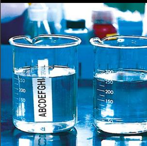
Glass plates with laminated labels attached were immersed in water and various chemicals for two hours. The text was unaffected.
