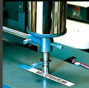
After a 1kg sanding device was passed over the laminated labels 50 times, the text was unaffected.
