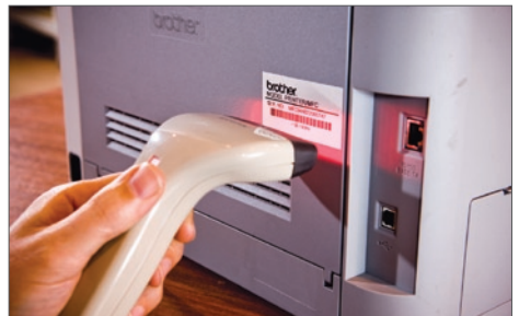
Connect a barcode scanner to the printer's serial port to print labels directly from the TD-4000/TD-4100N*
