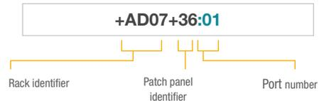
All ports on patch panels and all positions on termination blocks shall be labelled with the corresponding port number or position number and optionally with additional identifier fields as practicable.
