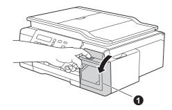
C Lift the cap of the ink tank for the colour you want to fill.
