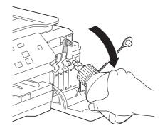
Push down on the cap of the ink tank to close it tightly.
