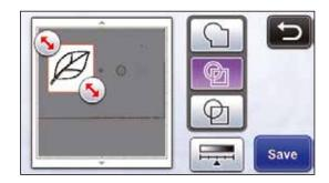
Use the touch pen to edit the image area for the cutting lines to be saved as data, and then touch the 'Save' key.
