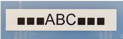
Label after testing: Label: Brother strong adhesive laminated TZe label Chemical: Acetone
