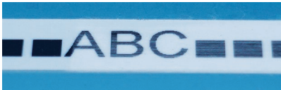
Label after testing: Label: Brother flexible ID laminated TZe label Test: Abrasion with sanding device
