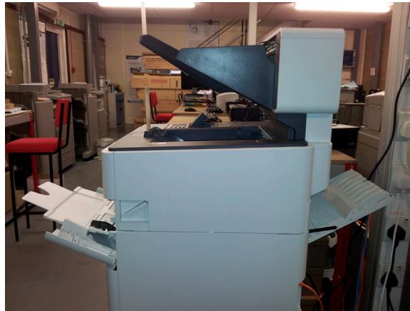
Straight paper route through device via multi-function input tray and rear exit tray
