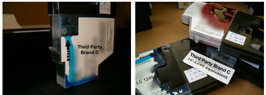
Ink leaked from the breather hole even when the cartridges were sitting vertically or lying flat with the breather hole upwards.
