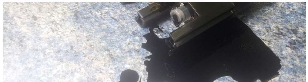
Black ink having leaked from black cartridge ink orifice after being removed from printer
