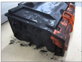
Eight cartridges from Brand G (examples shown above) experienced significant toner leakage right from the start. (Cartridges with this degree of toner leakage are considered out-of-box failures.)
