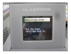
The first Brand K toner cartridge could not be recognized by the device, generating an error code upon installation.
