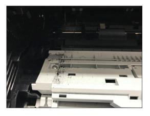
The printer using Brand F cartridges showed significant toner leakage on the manual feed tray, which could contaminate users' hands and pages with toner.
