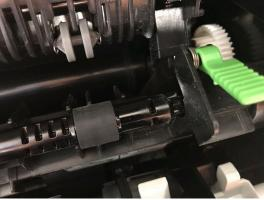
In the machine dedicated to Brother genuine toner (above left), the gear is clean and there is no sign of toner dust on the paper transport or the fuser entrance, above right; similarly, there is no evidence of toner dust at the back of the machine.
