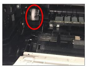
By the end of testing, a significant amount of toner dust had been deposited on the gear of the Brand H machine (above). Several other brands experienced similar build-up on the gears throughout testing.
