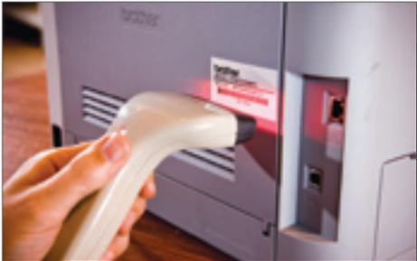
Connect a barcode scanner to the printer's serial port to print labels directly from the TD-4000/TD-4100N\*
